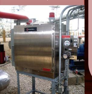
Parafuel<sup>™</sup> systems from LT Industries offer a *fast, accurate, easy and proven system for determining the point of asphaltene precipitation, crude oil stability* and other key properties in crude oil. Parafuel<sup>™</sup> systems are designed for use in both laboratories and the field. The analyzer can help you optimize process conditions to avoid asphaltene deposition in pipes and in the refinery, saving you time and money.
